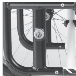
MA 114 Drive wheel adapter, permanently welded
