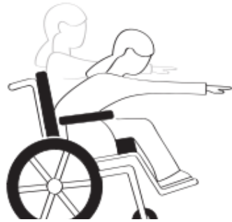
Figure 5.6: Forward reach in wheelchair
