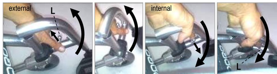
To swing the footplate frame externally, move the lever **L** sideward to same direction and turn the footplate frame.
