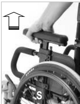
In order to check the correct position of use, with one hand, take hold of the armrest's pad and try to pull it up. If correctly locked, the armrest does not come off the support **S**, nor does the pad move up.
