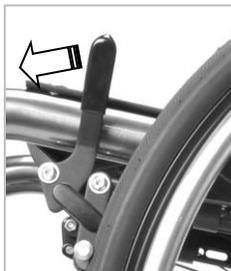
To engage the brake, pull the lever backward until it locks.
