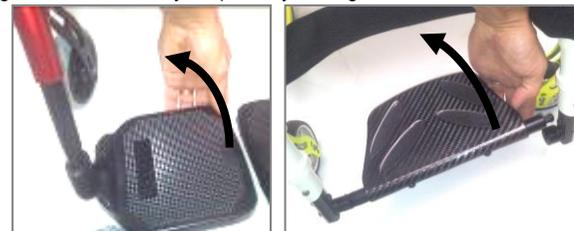
Flipping up the footplate is a very easy operation you can perform with one hand by pulling the plate up.
