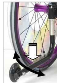
In order to check the correct position of use, with one hand, take hold of the tube and try to move it right and left: the tube should not turn (there may be a little play). Then, push the tube downward: the tube goes down by approximately 1 cm but it must not come off.
