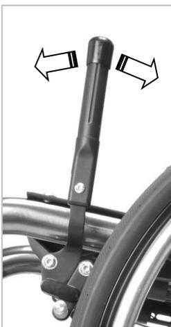
The brake (push-to-lock and pull-to-lock) with extended lever works in the same manner but results easier to engage and release.
