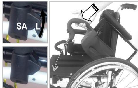
To remove the armrest, you have to swing it back first. Then, turn it until aligning the two marks **M** of the support **SP**. Only in this position, it will be possible to remove the armrest. Now, pull the armrest off.
