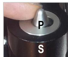
To remove the anti-tip wheel, push the pin **P** that is located in the upper side of the support **S** and push the tube down.
