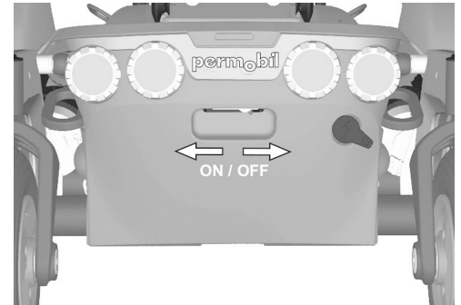
Figure 16. Main circuit breaker.
