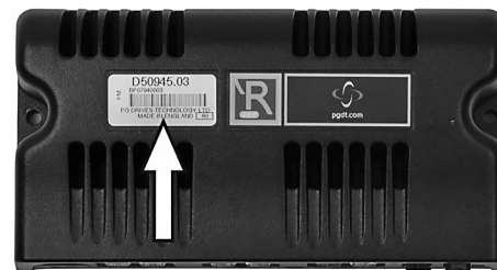
Figure 228. Power module ID number.
