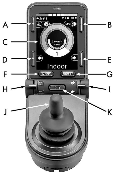
Figure 47. Control panel overview.
