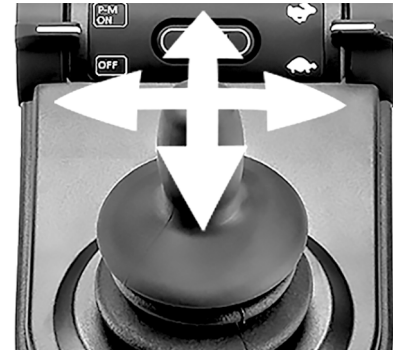
Figure 86. With the use of Bluetooth® the joystick can take control of the mouse functions.
