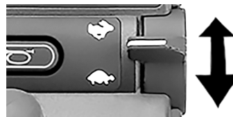
Figure 85. In mode Bluetooth® the right paddle switch is used to scroll up or down.
