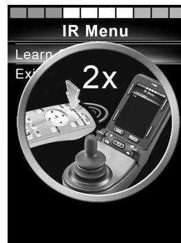
Figure 93. Point the remote control at the IR receiver. Press the button twice.
