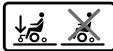
Figure 192. The support wheels must always be fitted when you drive.
