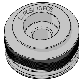
Figure 161. On top of the friction brake, there is a text that says either “12 PCS” or “13 PCS”.
