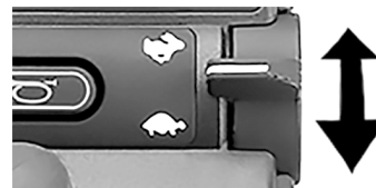
Figure 79. In mode Bluetooth® the right paddle switch is used to scroll up or down.
