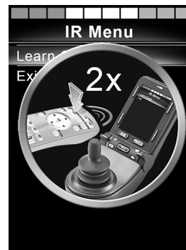
Figure 87. Point the remote control at the IR receiver. Press the button twice.
