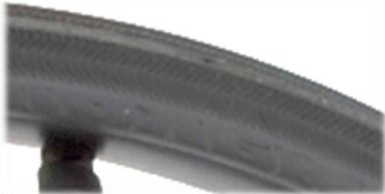
Solid tyre KIK MAKO Suitable for most environments, it does not need inflation, but it is less fluent, it has a little less grip especially over smooth and wet surfaces.
