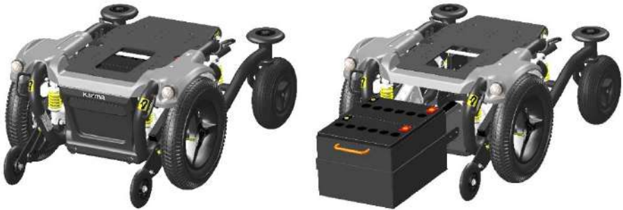
Position and access of the maintenance free batteries
