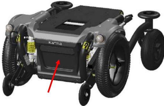
Position of the battery pole (behind the black cover)
