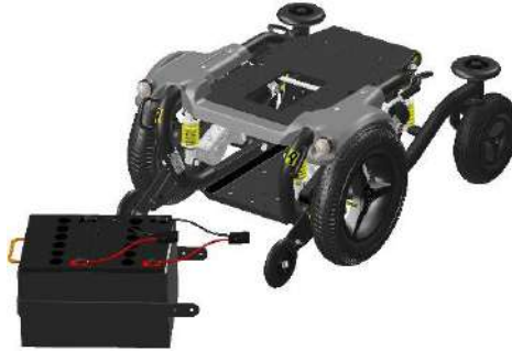
Unplugging the cables
