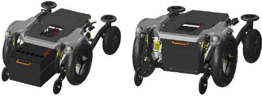
Placing the battery box into chassis and slowly slide in inside
