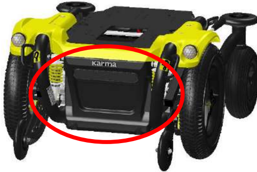
The front and rear battery box
