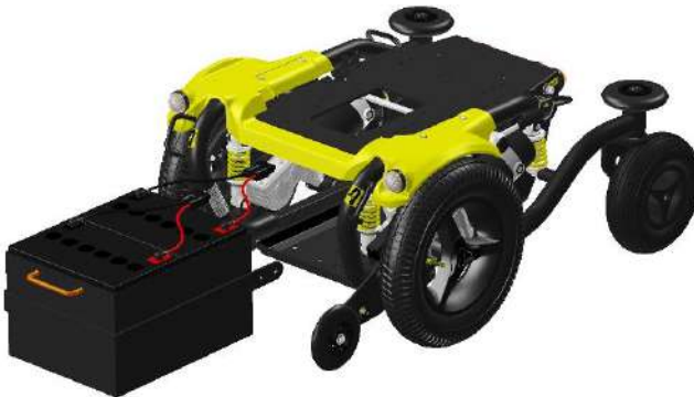
Battery box slides out of the chassis
