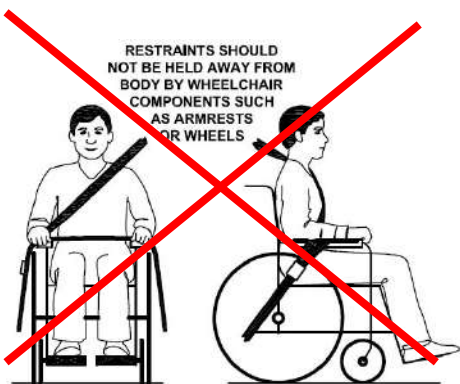
Picture of improper belt fit
