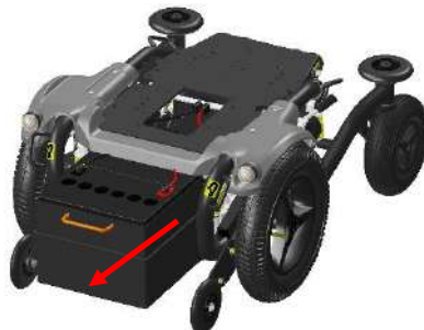
pulling out the battery box
