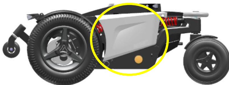
The battery box
