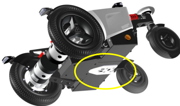
EVO chassis with Dahl Docking plate mounted.
