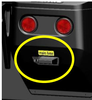
place of the main fuse
