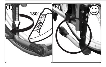
Only rotate the anti-tipper 180° from deactivated position to active position. Avoid full revolutions in one direction, since otherwise the tension spring inside the anti-tipper will be damaged, which may result in the anti-tipper losing its functionality.
