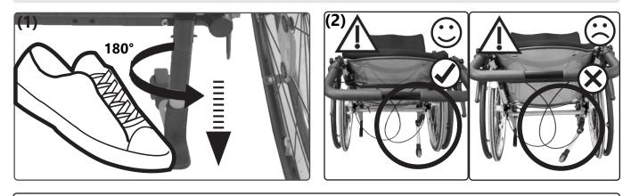
$m \uparrow$  The anti-tipper must always be locked in its end position.
