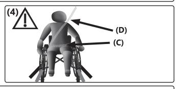
The seat belts must not be twisted during use, nor must they be guided over any structural components, which would keep them away from the body. They have to be tight and firm without impairing user comfort. The lap belt buckle must be positioned between the pelvic bones (if possible in the middle). The buckle tongues on the lap belt for fastening the shoulder belt should be located on the outside of the pelvis where possible.
