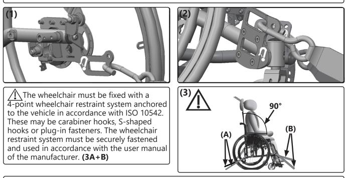
If the wheelchair is equipped with a back angle-adjustment or tilt mechanism, the occupant must sit in an upright position at a 90° back angle during transport (3). Leg supports that can be swung up must be adjusted to the lowest position.
