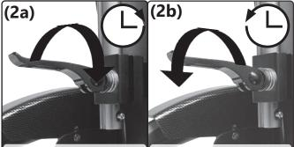
Increase clamping force Reduce clamping force
