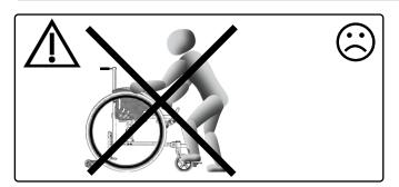
Do not use the footrest(s) for getting in and out of the seat shell-underframe, it may tilt forward.
