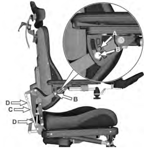
Figure 139. Adjusting the armrest height and angle.
