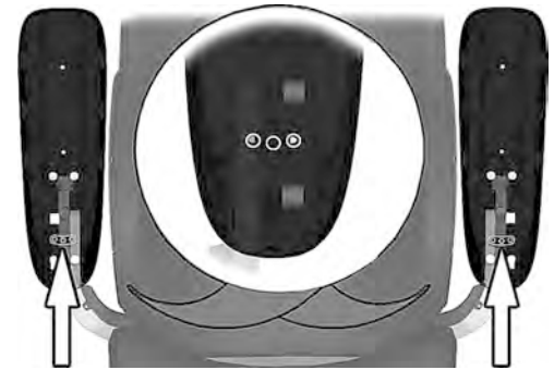
Figure 134. Adjusting the armrest rotation end position.
