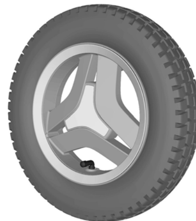
Figure 205. Filling valve on drive wheel.
