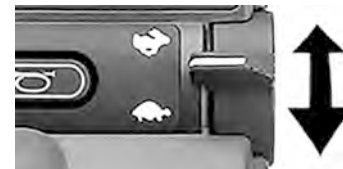
Figure 56. In mode Bluetooth® the right paddle switch is used to scroll up or down.
