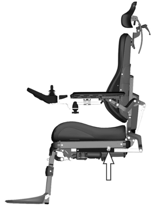
Figure 8. Manual clamping pole for the backrest recline.
