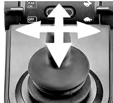
Figure 57. With the use of Bluetooth® the joystick can take control of the mouse functions.
