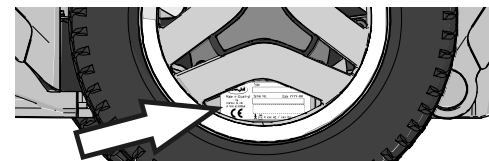
Figure 217. Chassis identification number label.
