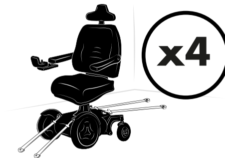
Figure 167. The wheelchair has four tie-down points. The wheelchair and tie-down position in this picture is generic.
