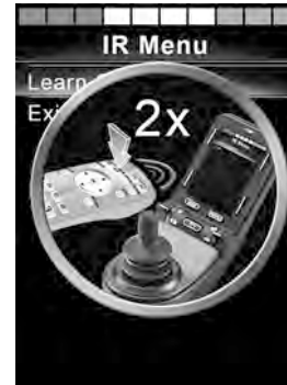
Figure 64. Point the remote control at the IR receiver. Press the button twice.
