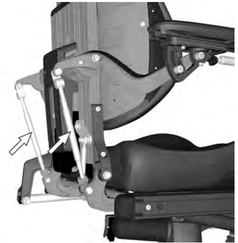
Figure 138. Armrest angle adjustment bars.
