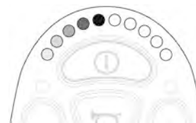
Figure 164. The LEDs on the battery voltage indicator.
