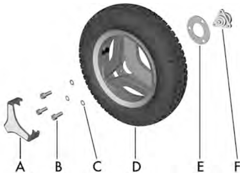
Figure 194. Installing the drive wheel.
