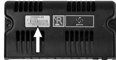
Figure 220. Power module ID number.
