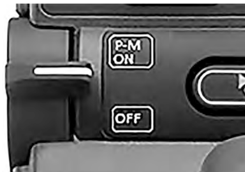
Figure 20. Power, mode and profile paddle.
