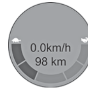
Figure 33. Maximum speed indicator.
