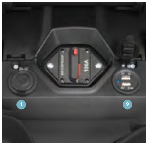
• 12-/24 V connection (1), USB charging receptacle (2)
