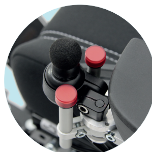
EU111 mo-Vis joystick incl. 2 finger button
