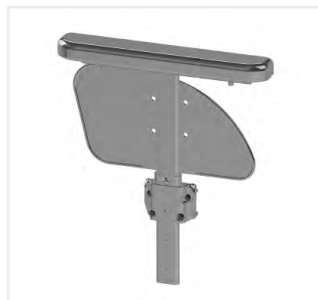
// QSC040052 Single-post sideguard, depth adjustable, tool height-adjustable
