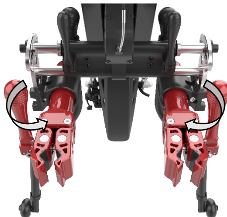
Figure 20. Reversing the Clamp Mechanism Receiver into inward orientation
