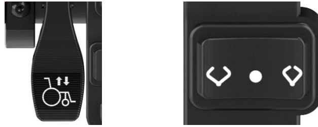
Figure 37. Manual Lift Lever and Auto Clamp/Lift Button
