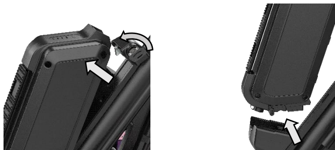
Figure 44. Removing and replacing the Battery.
