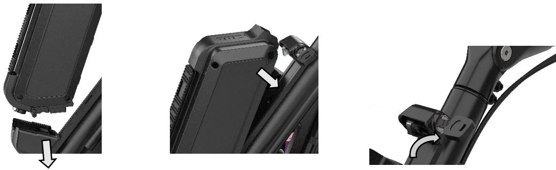
Figure 43. Inserting the Battery to the Battery Holder.
