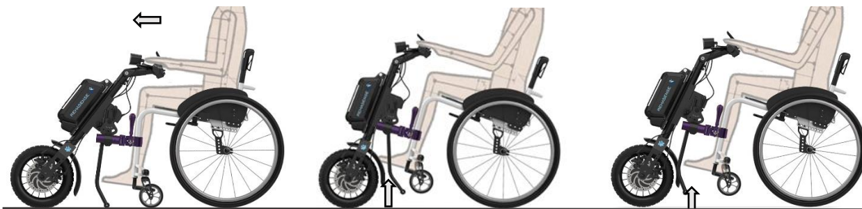
Figure 38. Parking (1), City (3) and Touring (2) positions for Manual Clamp/Lift Devices
