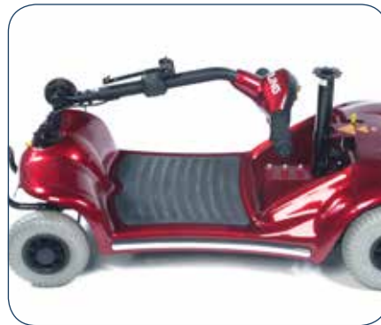
Easy to transport - when disassembled, the heaviest part of the Pearl weighs just 16 kg (35.2 lbs).
