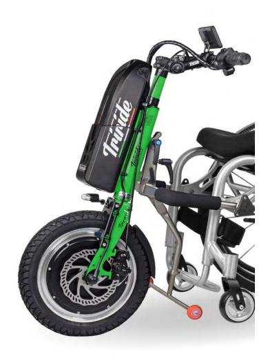
Superior power, with the motor integrated into the 14-inch rim, the L14 provides maximum performance for the most demanding users. . Great for tackling demanding situations, such as steeper inclines.
