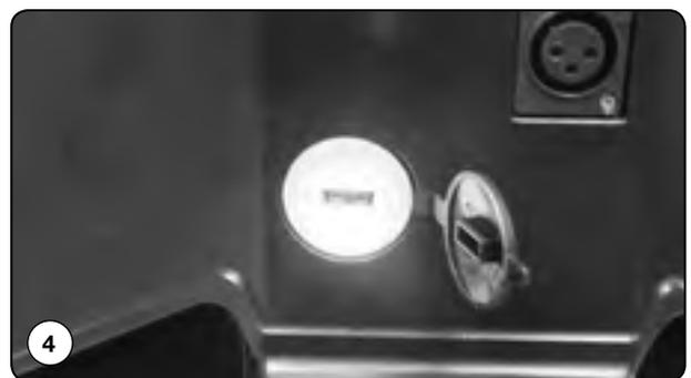
**Warning!** Never connect a device to the USB socket with a current rating of more than 3 Amps as this may cause the system fuse to operate.
