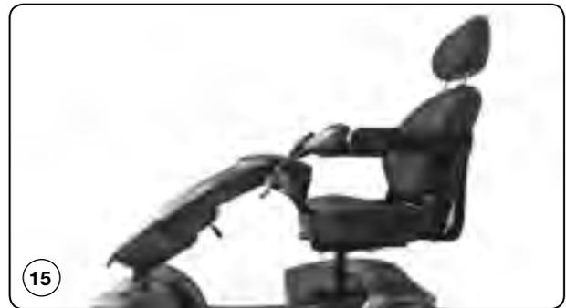
**Warning!** Before driving, always check that the tiller is securely in the upright driving position. Safe steering may be impossible if you do not !
