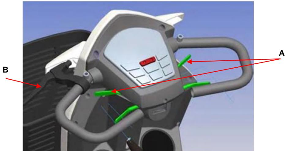
**A. Throttle Controls** – The Throttle Controls adjust the speed of your Vita Lite. The further you pull/push the control the faster your Vita Lite will go.
