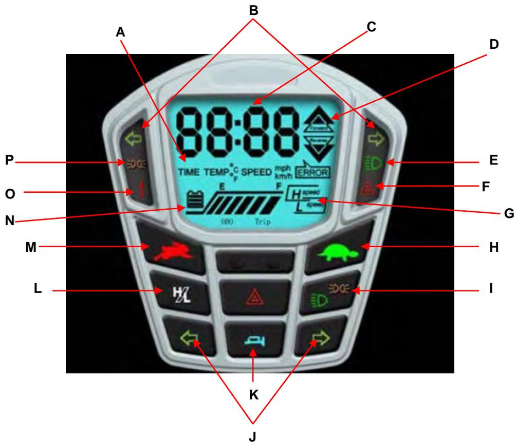
**A. Display Type Indicator** – The relevant light will illuminate indicating that the numerical display (C) above is indicating either time, temperature or speed.
