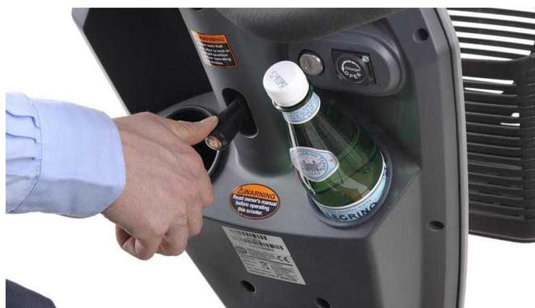
If you'd like to adjust the height of your Vita Lite tiller simply push the adjustment lever down towards the floor until the tiller moves freely up (away from the seat) and down (towards the seat). Once the tiller is in a comfortable position simply let go of the lever.
