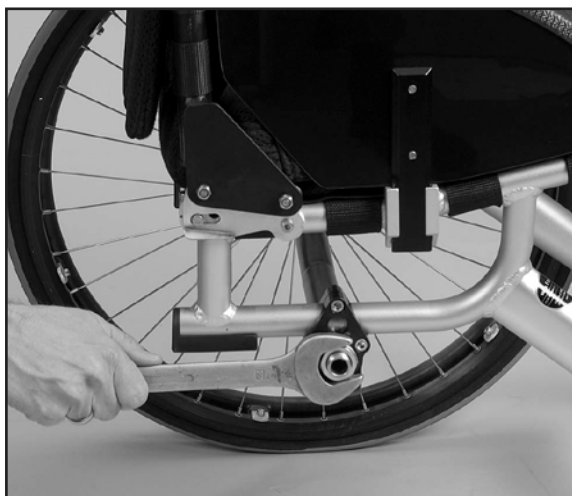
Image 36 Loosen the nut
