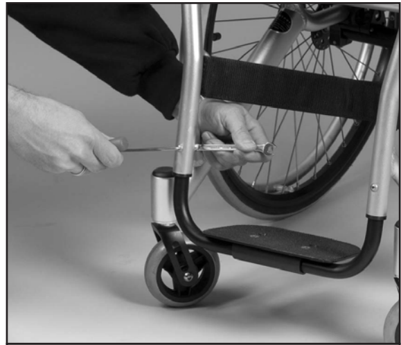
Image 28 Mount the nuts and bolts
