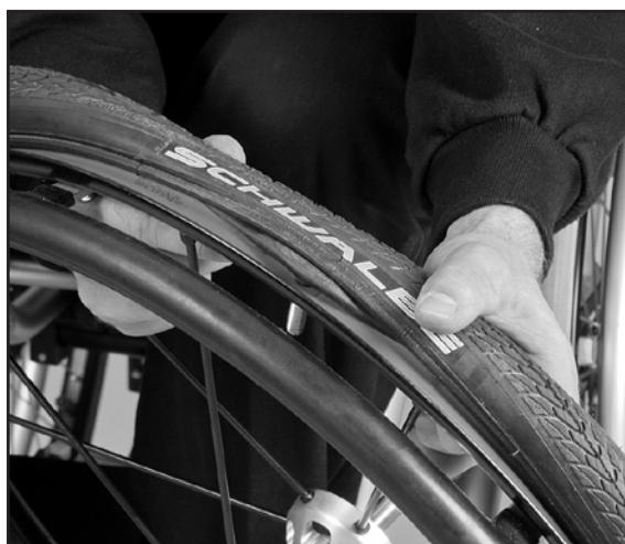
Image 48 Pull out the tube
