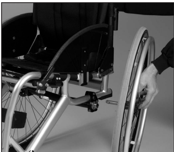
Image 23 Remove the rear wheels
