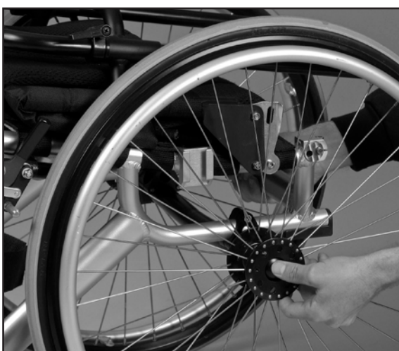
Image 6 Remove the rear wheels
