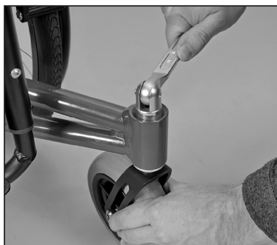
Image 39 Screw the nut off
