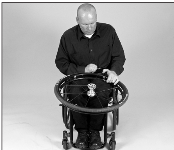
Image 47 Pull the tire edge over the rim
