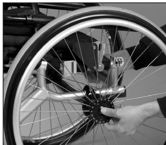
Image 26 Mount the rear wheels
