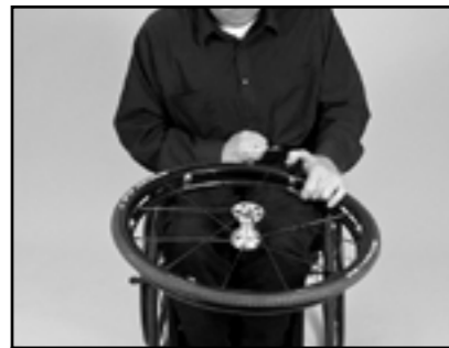
Image 68 Pull the tyre edge over the rim
