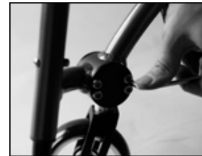
Image 55 Remove the four bolts
