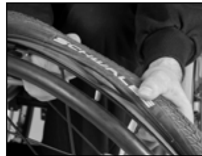
Image 69 Pull out the tube
