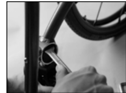
Image 56 Loosen the nuts
