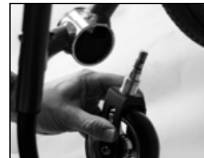
Image 57 Change the caster with front fork
